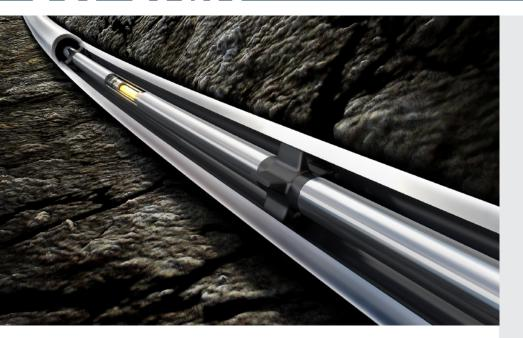
Scientific Drilling's Sci-GAIN™ is an API calibrated sensor that provides radial gamma ray and precision inclination measurements. On the Bottom Hole Assembly (BHA), Sci-GAIN is extended and positioned directly above the mud motor - giving gamma and inclination measurements that are closer to the bit than standard MWD measurements.
