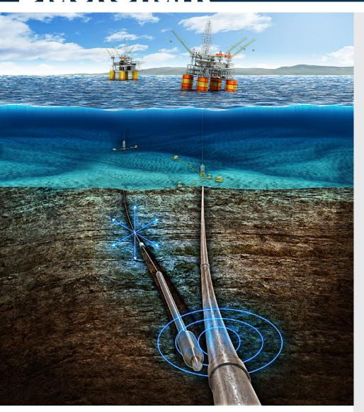
Scientific Drilling's BlackShark Active Ranging System is designed to deliver first-attempt relief well intersection, eliminating the need for costly and time consuming side-tracks.
