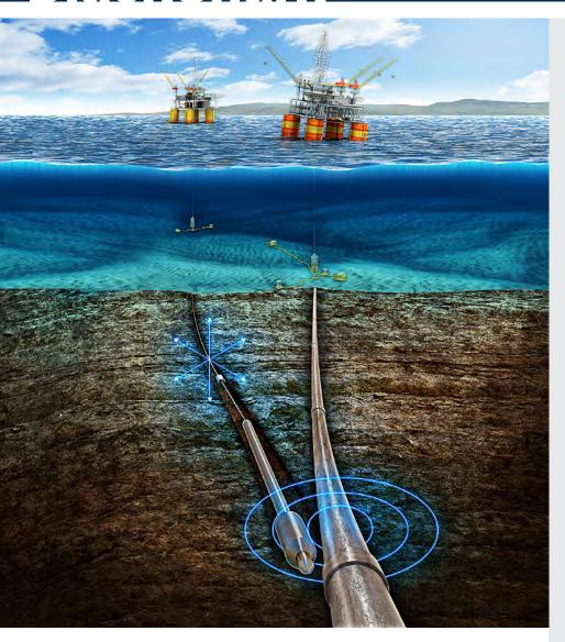
Scientific Drilling's BlackShark Active Ranging System is designed to deliver first-attempt relief well intersection, eliminating the need for costly and time consuming side-tracks.
