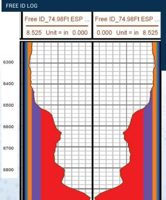
The Free ID represents the free space inside the (9 <sup>5</sup>/<sub>8</sub>") casing for a given OD and length of ALS or BHA, i.e. 74.98 ft.
