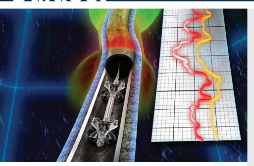
Scientific Drilling's DuraSet harnesses precise close interval survey data, collected by our high-speed Keeper gyro, with advanced 3D analysis software unveiling concealed wellbore tortuosity and determining the effective free ID, whilst computing bending loads along the entire length of the artificial lift assembly or other BHA.
