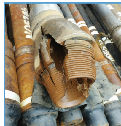
The last joint above the determined stuck point.
